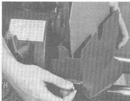
Figure 20. Move the guard cover towards the disc until it is approximately 1" away. Tighten both knobs.
