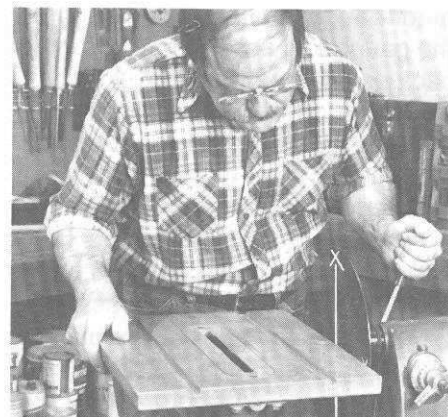
Figure 12. Checking the miter gauge slots.
