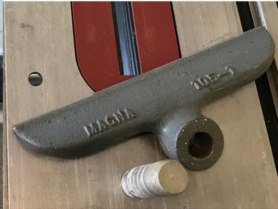
Headstock is in pretty good shape but bearings are stiff. Above is the Lathe Tool Rest with the screw in post.
