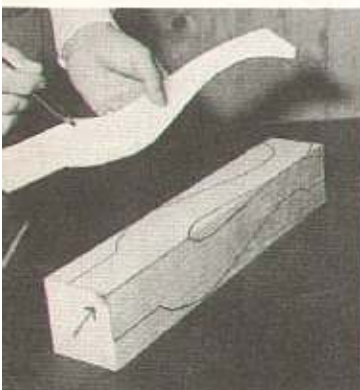
Cut the pattern with a long tenon piece. Mark the stock to identify the inside corner to avoid confusion later.
