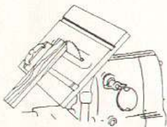
FOR BEVEL CUTTING, SET TABLE AT ANGLE REQUIRED AND MITER GAUGE AT 90°
