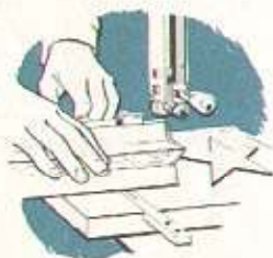
Duplicate pieces can be produced by pre-shaping a large piece and then resawing, like these stars.
