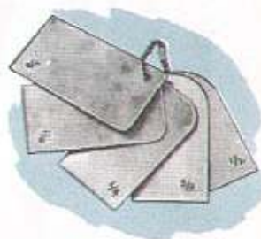
A set of aluminum templates is handy to determine the minimum turning radius for each width of blade. Patterns above are actual size for each blade size.
