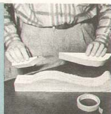
Save the waste stock: it must be replaced on the cut to provide bearing surface. Two-faced Scotch tape works well.
