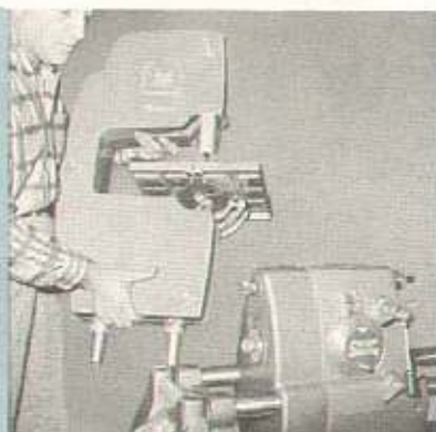
Mount band saw on Shopsmith using Power-Mount and flexible coupling, or on stand as single-purpose tool.
