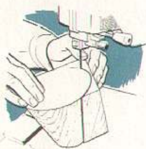
Circular cuts with the table tilted produce cone-shaped blocks, reducing lathe work.
