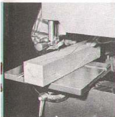
Now make the second cut with the first face against the table. Again, replace the pieces you have cut out.
