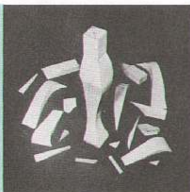
And there you are: the cabriole leg emerges from the block, ready for final smoothing and sanding and finishing.
