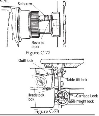
When changing from a horizontal to a vertical position, secure the base lock. When changing from vertical to horizontal, secure the power mount and base mount knobs. If you're mounting accessories in the power mount or base mount, secure the mount locks.
