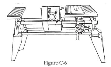
**13**. With the machine setting upright securely tighten all ten screws and nuts that hold the legs to the headrest and bench.
