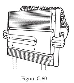
rock the table. This will position the support tubes at exactly the same height and get the racks started properly in the pinions. Lower the table, loosen the tilt lock, set the desired position and secure the tilt lock.
