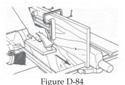
Use a push block to feed the workpiece from back to front, because the bottom of the bit is doing the cutting.
