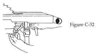
**27.** Loosen the tilt lock, move the worktable, then depress the 0° stop pin until the stop bolt contacts it. Tighten the tilt lock, and recheck the setting by repeating Steps 24 through 26. See Figure C-33. (It is very important to recheck the setting!)
