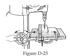
**4.** To position the table assembly on the way tubes, hold the carriage so that it won't drop against the base mount, then loosen the carriage lock. Adjust the table height so that the tip of the drill bit is 1/4"-1/2" above the stock, and tighten the lock.
