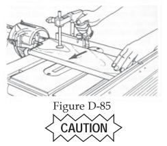
When using the miter gauge in the left slot, position the table so that the miter gauge clears the bit.
