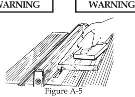
Use the fence straddler to hold down and push stock narrower than 1-1/2" past a blade or cutter. The body rides on the rip fence, while the heel hooks over the back edge of the stock. To change the height of the heel, loosen the locking knob. To reverse the heel, rotate the side 180°. Keep the locking knob secure. See Figure A-6.
