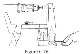
b. To adjust the cup center point vertically, loosen the mount lock, then loosen the tailstock stop collars. Raise or lower the tailstock in the base mount until the cup center point vertically lines up with the drill chuck, then tighten the mount lock. Press the stop collars down firmly against the base mount and tighten the collar set screws, as shown in Figure C-76.
