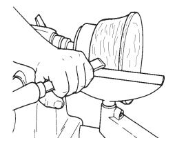
a. Scraping is one way to shape the inside. Turn on the machine, set the speed, and feed a roundnose chisel against the downward side of the stock. See Figure D-53. As you work, periodically check the inside diameter with inside calipers.
