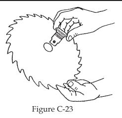
**b.** Hold the blade with the teeth pointing toward you, as shown in Figure C-23, then insert the arbor through the hole. Replace the nut and finger tighten it, as shown in Figure C-24.
