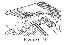
a. Use a long Allen wrench to loosen the lock knob (268) and adjust the miter gauge so it is perpendicular to the saw blade, then tighten the lock knob<sub>1</sub>. See Figure C-51.
