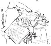
Figure D-14 Cutting a Compound Miter
