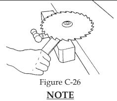
The only time the saw blade is used without the upper or lower saw guards is during alignment and only after the Mark 7 is turned off and unplugged.
