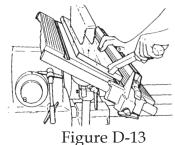
When ripping a bevel in stock narrower than 1-1/2" wide, you'll need to mount an appropriately thick piece of stock to the rip fence. This fence extension will position the ripping face closer to the blade for narrower cuts.
