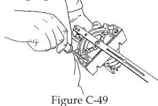
**c.** Return the miter gauge to the slot and recheck and readjust it, if needed.
