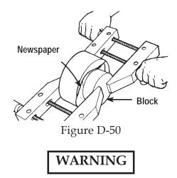
If the screws are being driven into end grain, the screws must sink into the block at least 2". Use #12-by-2 1/2" long wood screws.
