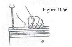
8. Attach each feather board holder to the shaper fence, see Figure D-66.
