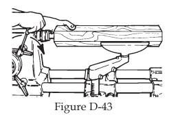
**f.** Adjust the height of the tool rest and align it parallel to the stock and not more than 1/4" away.
