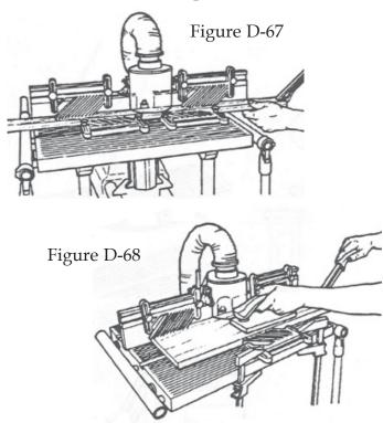
Figure D-68 illustrates two feather boards mounted on a feather board holder. Since the workpiece is too wide to install a feather board in the miter gauge channel of the worktable, notice how the horizontal feather boards is clamped to the worktable. When you want to use feather boards for horizontal pressure on the workpiece, remove the channel guide from the feather boards and clamp the feather board to the front of the worktable. Using the Miter Gauge with the Shaper Fence
