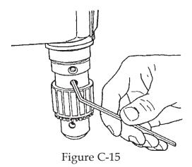
**9.** Install a 3/8" to 1/2" straight drill bit in the drill chuck and use the chuck key to lock it place. See Figure C-16.
