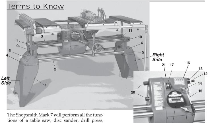
tions of a table saw, disc sander, drill press, horizontal boring machine, wood lathe, overtable router, and under-table shaper.
