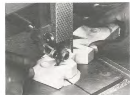
Figure 11. To cut corners and curves in tight spots, feed the wood very lightly against the blade and let the teeth nibble away the stock.
