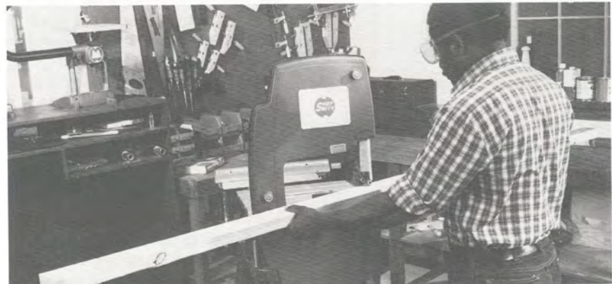
Figure 13. With the blade offset, you can crosscut long boards, up to 3-7/8" wide.
