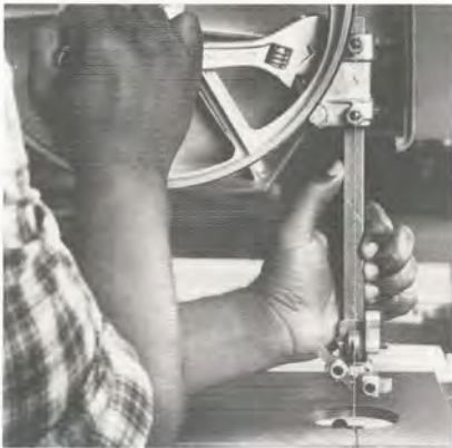
Figure 11. To adjust the upper blade guide roller side-to-side, loosen the two guide post retainer mounting bolts, pivot the upper blade guide sideways until the blade is centered on the roller, and tighten the bolts.
