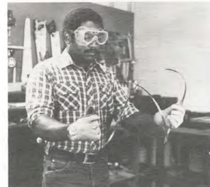
Figure 12. Rotate your hands in opposite directions. The blade will begin to coil back on itself a second, and then a third time.
