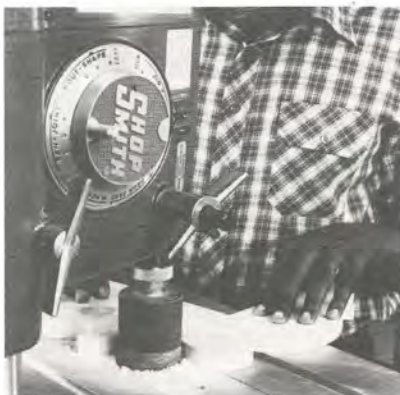
Figure 5. For smoothness and accuracy, cut outside the pattern line in the waste stock, then sand the workpiece to the final dimensions.
