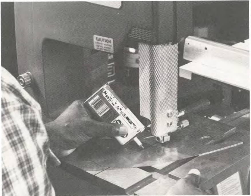
Figure 26. When cutting hard materials, slow the speed of the bandsaw and the feed rate down. Apply oil to metals to help keep the blade from overheating.
