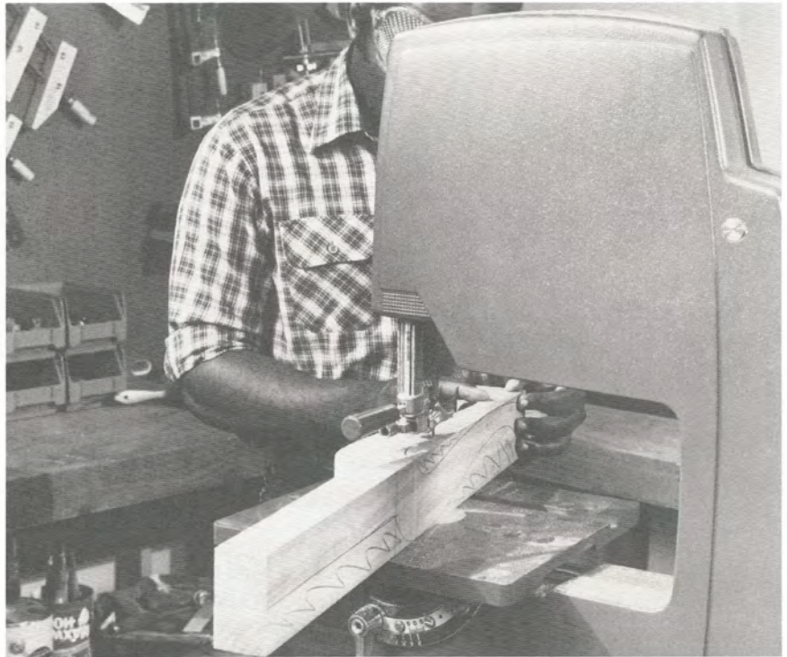
Figure 23. To make a compound cut, begin by cutting a pattern in a workpiece as you would normally, but save the waste.
