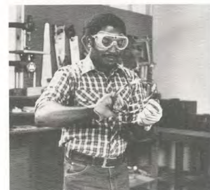
Figure 13. Let the coils fall into place naturally as you turn your hands. When you have rotated each hand 180°, the blade will be completely coiled.
