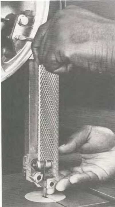
Figure 13. To adjust the tension on the upper blade guide height lock, turn the adjusting screw on the left side of the guide post retainer.
