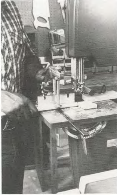
Figure 20. Use the miter gauge or V-block to crosscut round stock. By attaching a stop block to the left side of the table, you can accurately cut duplicate lengths.
