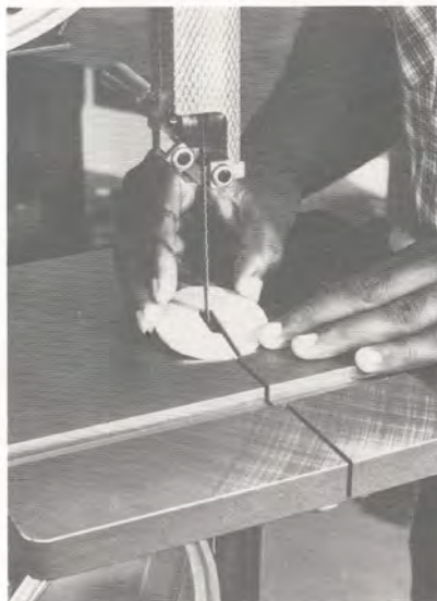
Figure 8. Install the table insert so that the key fits into the split in the table.
