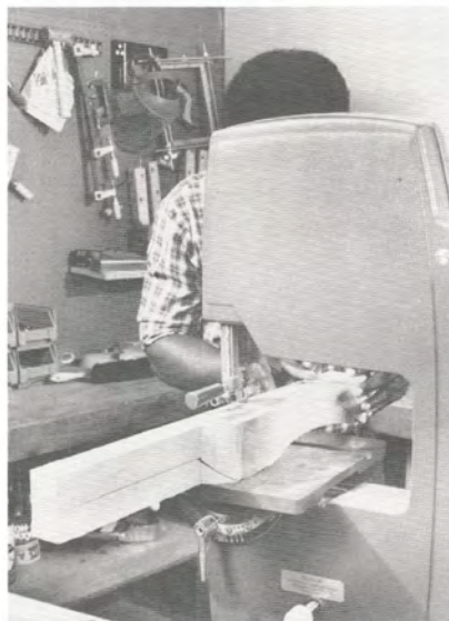
Figure 24. Tape the waste stock back to the workpiece and make another cut.
