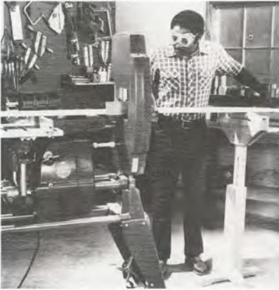
Figure 8. With your bandsaw mounted on the Mark V, you can use the Mark V table and rip fence for additional support.
