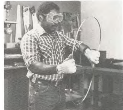
Figure 11. To coil a bandsaw blade, hold it out in front of you with both hands. The palm of one hand should face in, the other should face out.
