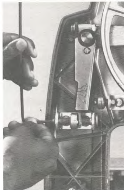
Figure 4. With the blade in position, turn the tension screw clockwise until the scale indicates the correct tension for the width of the blade being used. As shown, the tension is properly set for a 1/4" blade.
