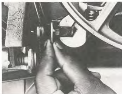
Figure 9. To adjust the auto-track roller, loosen the mounting bracket bolt and slide the bracket sideways until the roller is centered behind the blade. Keep the roller parallel to the blade when you tighten the bolt.
