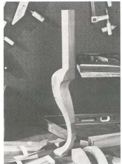
Figure 25. When you remove the waste, you'll have a piece that looks handcarved, like this cabriole leg.
