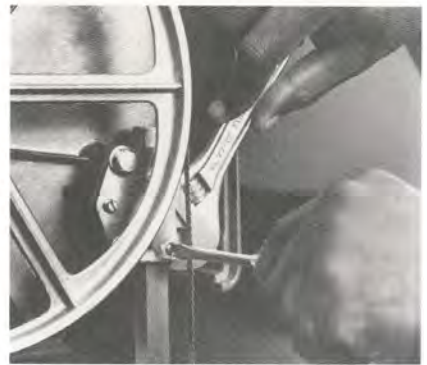
Figure 12. To adjust the upper blade guide roller front-to-back, loosen the jam nuts on the two guide post adjusting screws. Turn the screws until the roller is properly positioned, then tighten the jam nuts while keeping the screws from turning, as shown.
