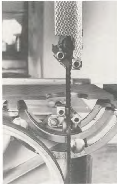
Figure 20. By reversing the guide blocks, you can offset the blade 30° to the right. This allows you to cut off any length of stock without interference from the bandsaw frame, as long as the stock is not more than 3-7/8" wide.
