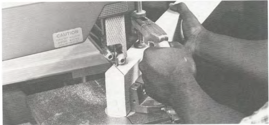
Figure 12. By mounting the miter gauge in the table slot that runs parallel to the flat of the blade, you can crosscut and miter.
