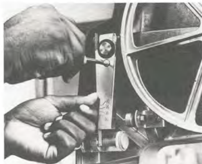
Figure 8. Realign the tension scale so that it's parallel with the indicator bar, as shown.
