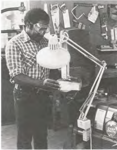
Figure 3. To provide a concentrated beam of light when doing fine work, mount an inexpensive drafting lamp to the Mark V way tubes.
