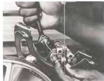
Figure 10. To adjust the lower blade guide roller, loosen the mounting bolt at the back of the bandsaw. Slide the assembly sideways until the roller is centered behind the blade and then tighten the bolt.
