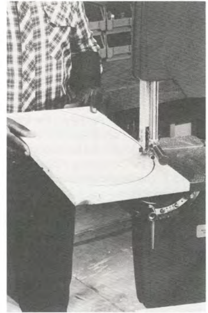
Figure 4. The same cut that was shown in Figure 3 should have been started as shown here in order to complete it successfully.
