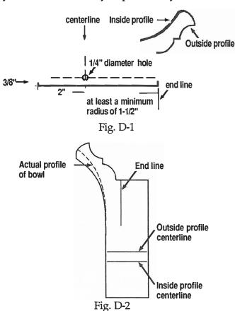
To cut both profiles without remounting the stock, there may be times when you'll need separate internal and external templates. This will be determined by your setup, the optional accessories you're using and how the stock is mounted to the faceplate.
